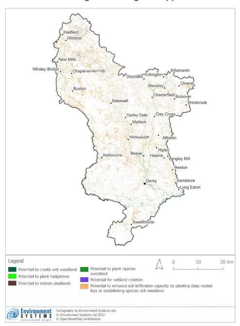
This map was made from the full map of NFM opportunities. It is a selection of areas that occur in the places that have a high hydrological conductivity, meaning the most significant locations for funnelling water towards the rivers and streams. Areas of high hydrological connectivity were identified by analysis of the Digital Elevation model with SCIMAP.
