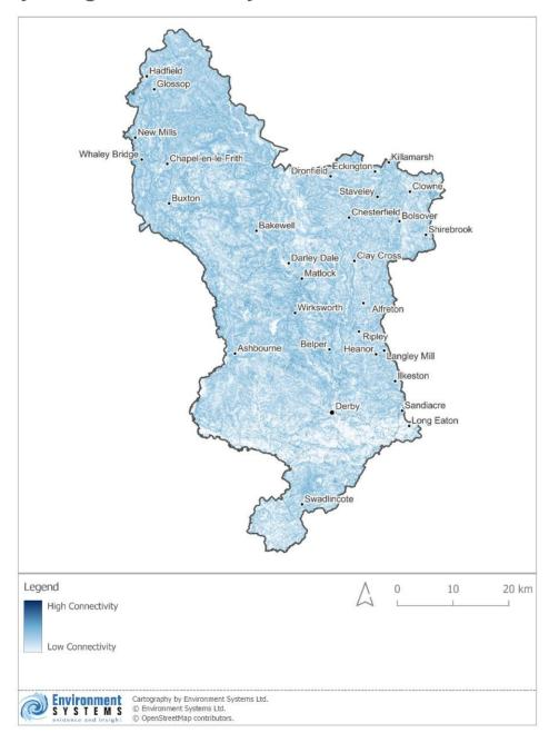
This map shows how strongly areas are connected to the channel network; how important each location is for funnelling water towards the rivers and streams. Areas with high
